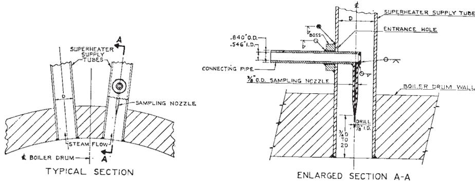
NOTE 1—Sampling nozzle shall be centered on superheater supply tube.
