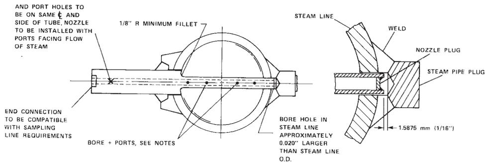
NOTE 1—The design, materials, construction, welds, heat treatment, and non-destructive test requirements shall be in accordance with all applicable codes. The dimensions given are only a guide and should be checked for each case.
